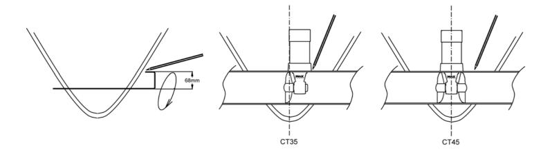
Replace the tunnel. To secure its position apply reinforced fiberglass filler to all areas, both inside and out, taking care to entirely fill the space between the hull and the tunnel. Laminate using a minimum of 8 layers of **ISOPHTALIC RESIN** alternated with mat and roving.
