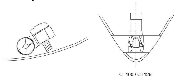
propellers of either models protrude out of the tunnel.
