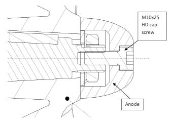
6) Insert the anode on the shaft. The anode in centered by the washer M20. Then screw the hd cap screw M10x25 on the propeller shaft putting on the thread of the screw a few quantity of Loctite 243 medium grade.
