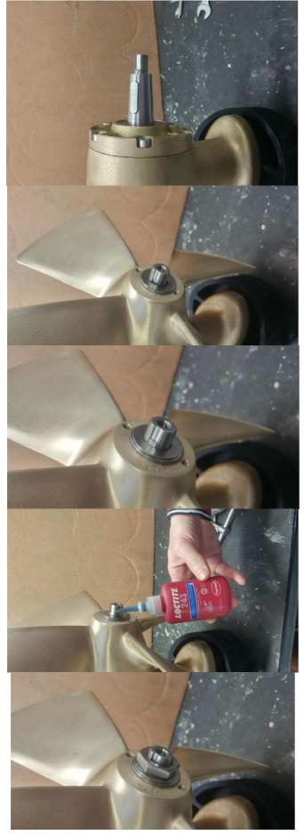
1) Insert the key into the keyslot of the propeller shaft
