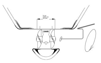
Fit the tunnel and mark the areas to be fibre-glassed. Sand these areas inside and out.
