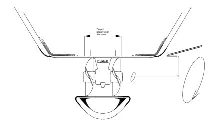
Fit the tunnel and mark the areas to be fibre-glassed. Sand these areas inside and out. In certain installations it is preferable to drill the position of the thruster support before the installation of the tunnel.
